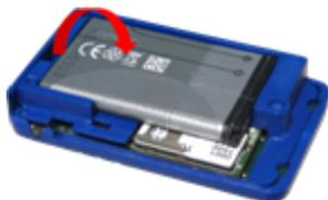
The PERGO package contains 1 rechargeable Li-ion battery. This battery must be installed as shown in the figure by opening the rear lid, placing the battery and closing the lid.
