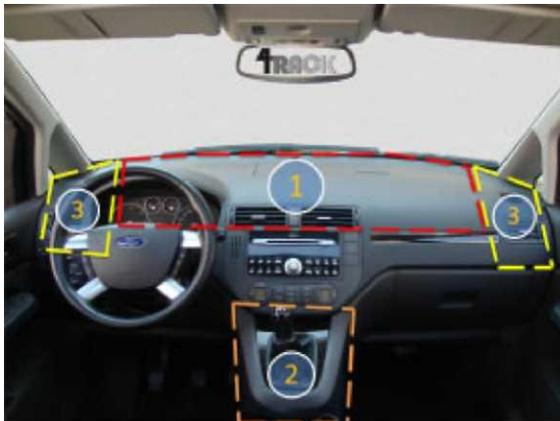
The correct operation of the installed device depends entirely on the place of installation. To ensure that the GPS module within the device is able to obtain a location fix, the device must be installed making sure that the logo on the device box in the shape of a satellite dish faces skywards.
